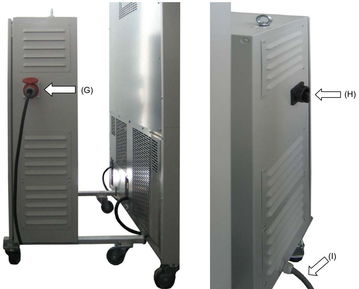
Left side of the voltage and frequency changer with connection socket (G) for the alternating climate chamber
